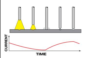
The wire is fed at a rate which is just greater than the burn-off rate for the particular arc voltage being used, as a result the wire touches the weld pool and short circuits the power supply. The filler wire then acts as a fuse and when it ruptures a free burning arc is created. This phenomenon is repeated regularly up to 200 times every second.
