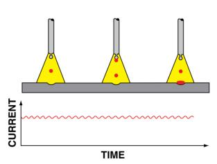
This mode of transfer consists of a 'spray' of very small molten metal droplets which are projected towards the workpiece by electrical forces within the arc. This mode of transfer is particularly suited to 'downhand' welding, but can be used by positional welding with aluminium and its alloys.
